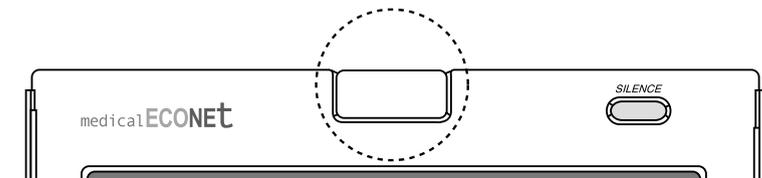
The LED located on the top of the front face Panel displays Alarm and Heart Rate Rhythm.
