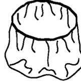
The intermediate filter should be replaced with every fifth change of paper bag and whenever there is damage or a visible collection of debris on the outside of the filter.
