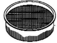
Replace the HEPA filter when loss of vacuum continues to occur after you have checked for an obstructions in the hose or wand. Also, install a new disposable paper bag and intermediate filter.
