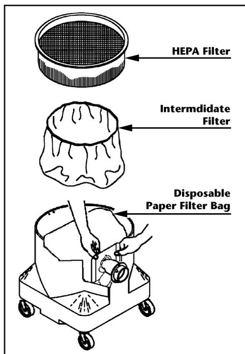
The intermediate filter is a very fine non-woven filter that extends the life of the expensive High-Efficiency Particulate Air (HEPA) filter.
