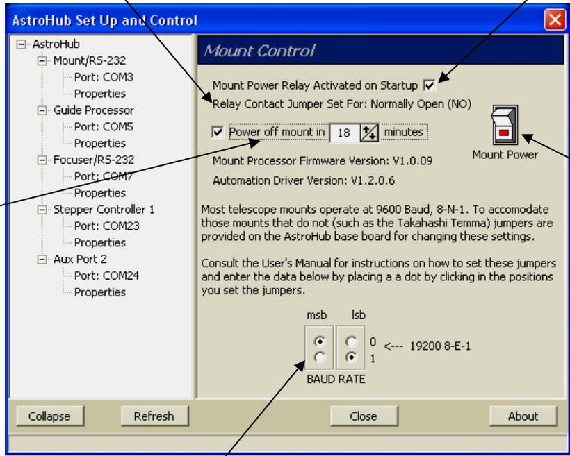
Mount communication parameters jumper settings found by the set up program. Assure the jumpers are set to match your mount. Change them here if you change them on the base board
