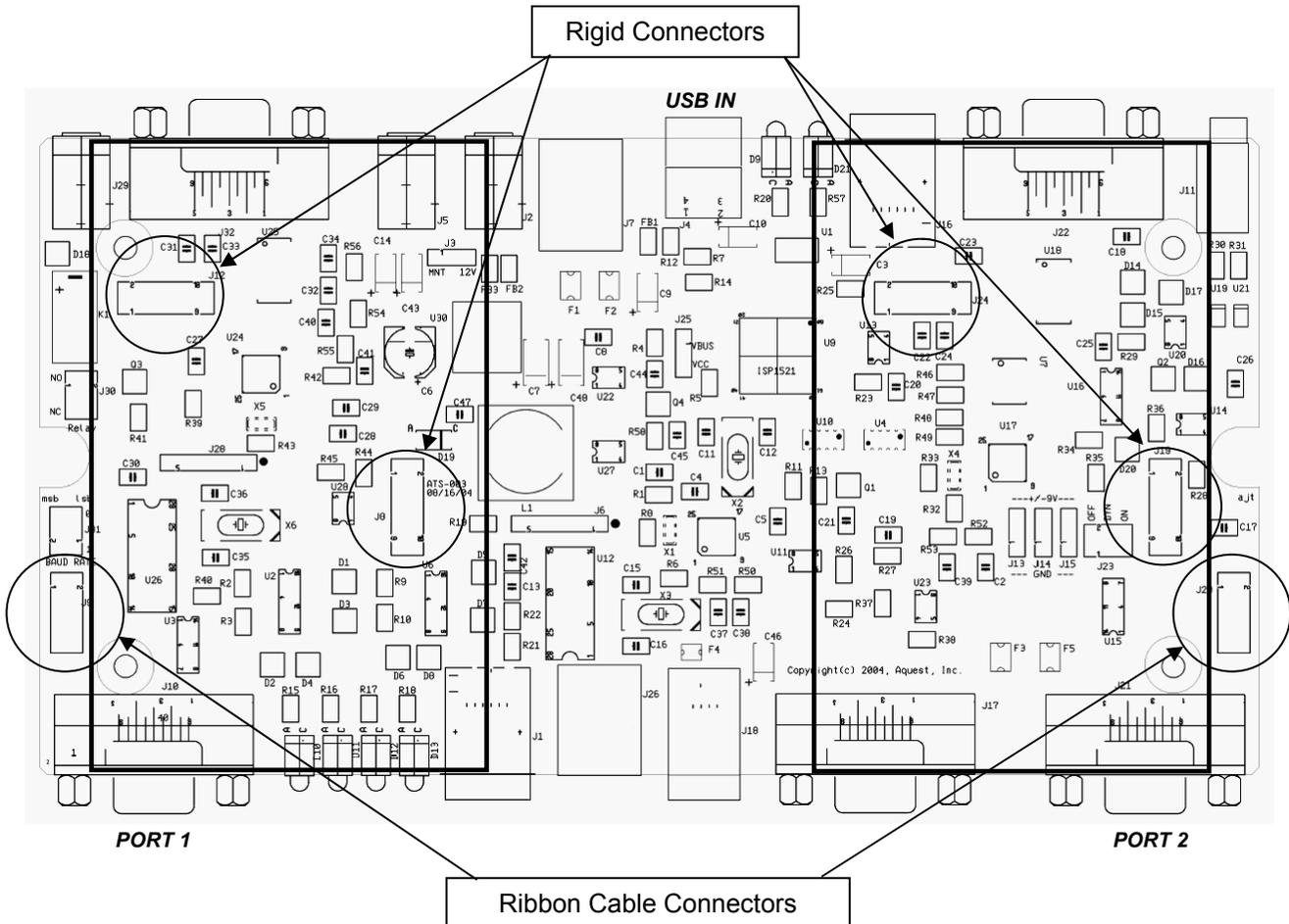
The Port 1 external connector and part of the Misc. Port connector are associated with Plug-in 1 and Port 2 and the rest of the Misc. Port connector are for Plug-in 2.
