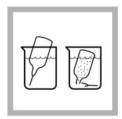
**5.** Fill a DPD Free Chlorine Reagent AccuVac Ampul with sample. Keep the tip immersed while the Ampul fills completely.
