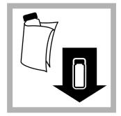
**3.** Wipe the blank and insert it into the cell holder. **ZERO** the instrument.
