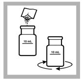
one DPD Free Chlorine Powder Pillow to the prepared sample cell. Swirl the sample for 20 seconds to mix.
