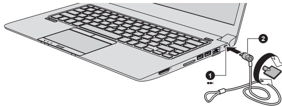
Figure 4-14 Security lock (Z30-B)
