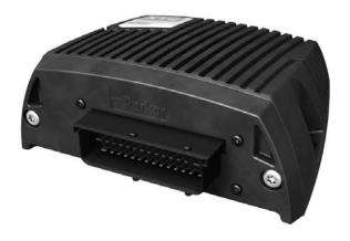
Weight 0.7 Kg -40 to +70 °C Operating temperature Protection outdoor use Voltage supply 9 - 34 VDC Current consumption (idle) 105 mA (28 VDC) 90 mA (14 VDC) Data interface Parker ICP (IQAN CAN Protocol)
