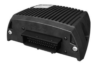
Weight 0.7 Kg -40 to +70 °C Operating temperature Protection outdoor use 11-32 VDC Voltage supply Current consumption (idle) 180 mA (28 VDC) 170 mA (14 VDC) Data interface Parker ICP (IQAN CAN Protocol)
