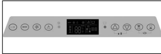
**I/O Power Switch:** Turns unit On / Off.
