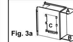
Rain hood inserts are installed in "A" and "B" positions with vent opening facing down (C)
