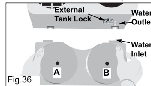
3. To make the connection, simply push the water tank down firmly onto the support hangers on the back of the cabinet and the water tank support tray.
