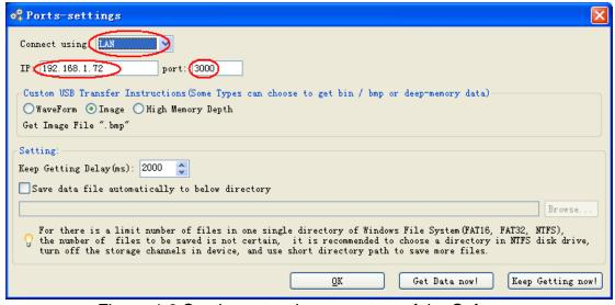
Figure 4-6 Set the network parameters of the Software
