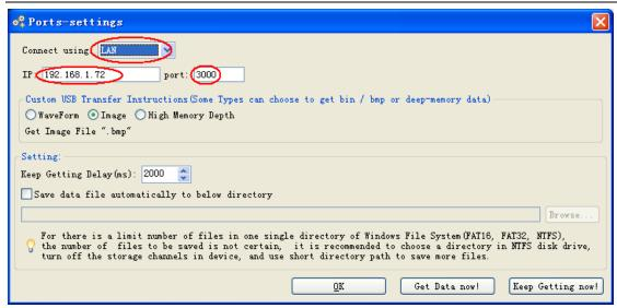
Figure 4-3 Set the network parameters of the Software
