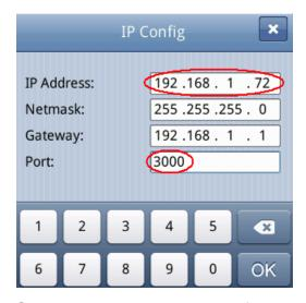
Figure 4-4 Set the network parameters of the oscilloscope
