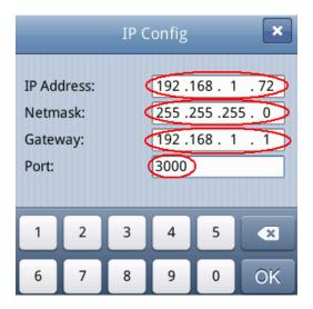
Figure 4-7 Set the network parameters of the oscilloscope
