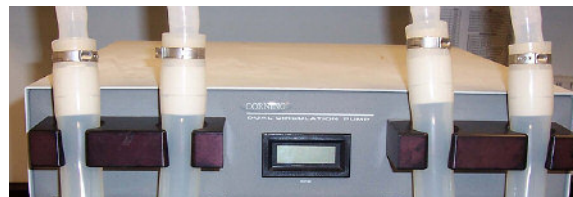
Figure 35. Installing the Dual Circulation Pump Cassette, Top View
