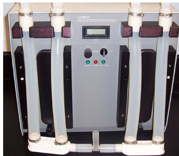
Figure 36. Installing the Dual Circulation Pump Cassette, Total View
