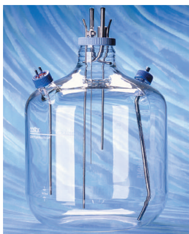
Figure 7. 36L Oxygenator (Corning Cat. No. 9979)
