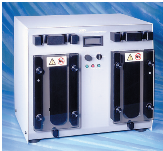
Figure 33. Dual Circulation Pump (Corning Cat. No. 3223)
