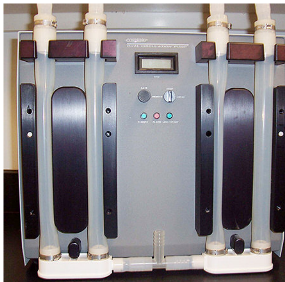
Figure 38. Installing the Dual Circulation Pump Cassette, Complete
