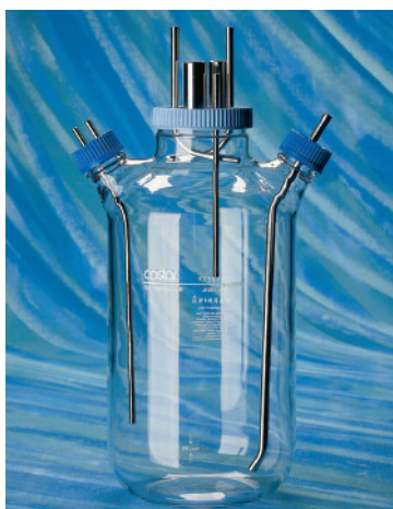
Figure 6. 6L Oxygenator (Corning Cat. No. 9983)
