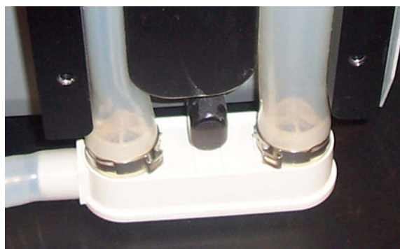
Figure 37. Installing the Dual Circulation Pump Cassette, Bottom View
