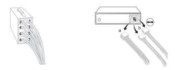
Starting from the black 24-pole Molex connector (connector 1, which is plugged into connection 2 on the electronics box), you will find one yellow (radio muting) and one red (steady plus) cable with plug connectors with a 24-pole plug connector.
