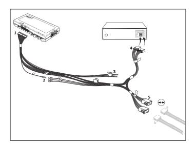
Three other cables are positioned opposite to the single yellow cable (2) for the radio muting. You can also find the correct cable here via Multimeter.
