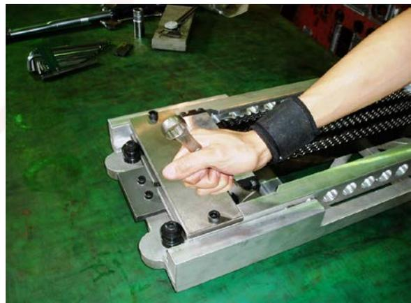
(2. Loosen the blades by pulling upward the handle in 90° )
