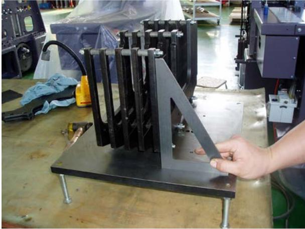
3. Calibrate the perpendicularity on the adjusting platform for the feeding base.
