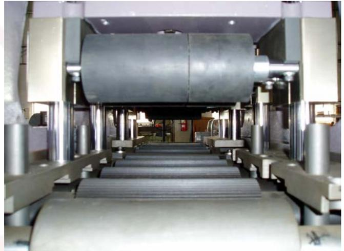
Replace method: Loosen the retaining screws M6 under the fixing plate of the pressing wheels, loosen the retaining screws for the pressing wheel slides, and take off the pressing wheels. Take off the snap rings with a snap ring plier and replace the snap rings.
