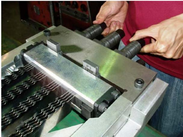
(4. Insert into the clearance with four 5mm shims, and then properly screw these three nuts with hands so that the clearance becomes 10mm. Withdraw the shims)
