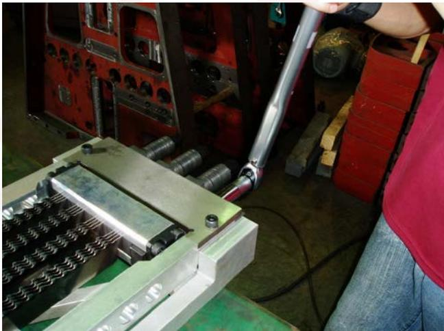
(10. Tighten the push bolts to 75Nm. Now the saw blades are fully clamped and unable to slide)
