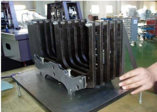
5. Calibrate the perpendicularity of the feeding base again.
