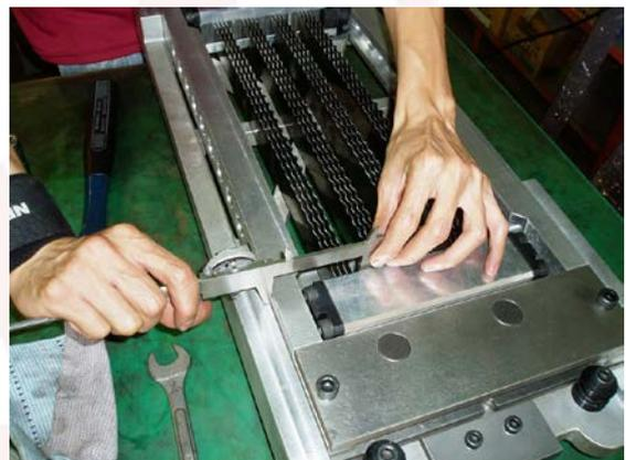
(13. The parallelism between the saw blades and the frame shall be kept below 0.05mm)
