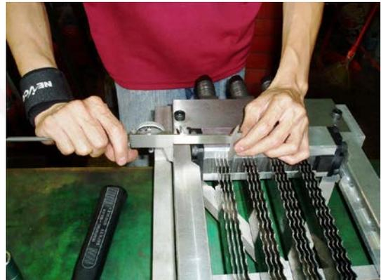
(12. Check the parallelism between the saw blades and the frame)
