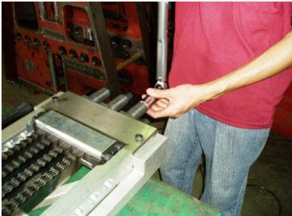
(Adjust the torque wrench to 120Nm)
