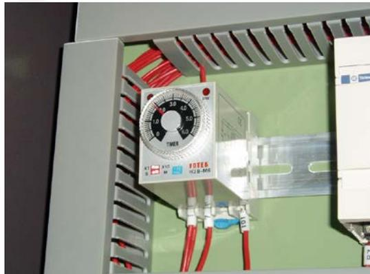
(This timer controls the oil supply interval. The factory setting of oil supply interval is once per 3 minutes. If the amount of oil is to be increased, the interval shall be shortened)
