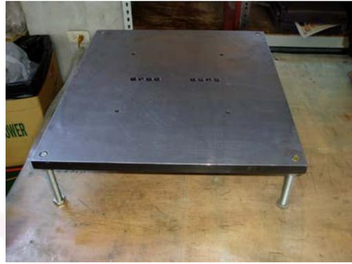
2. Mount the tool holder on the workbench (uneven workbench shall not be used for the torque is great when the frame is tightened)
