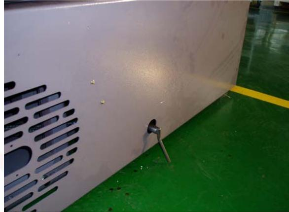
2. Install the frame and tighten the frame to 60Nm with a torque wrench. Withdraw the pin.
