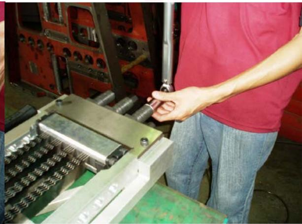
(6.1 Adjust the torque wrench to 60Nm)
