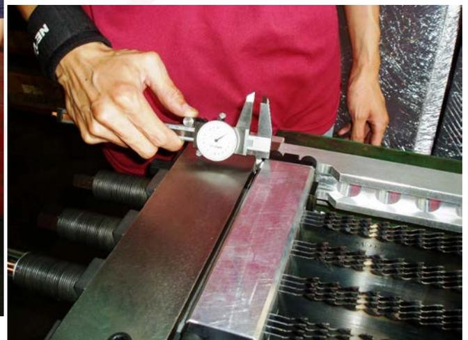
(8. The parallelism error of the clearance can be corrected with the three draw-in bolts)
