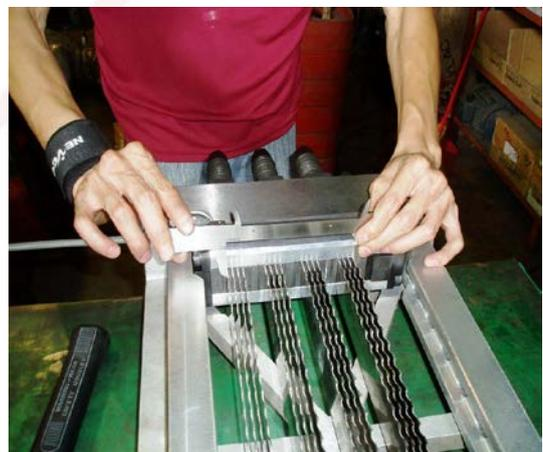
(14. Check the parallelism between the saw blades)
