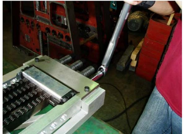
Loosen the push bolts, and knock the push bolts loose with a hammer.
