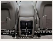
the device and plug it in again. To avoid overloading the circuit, check the power ratings on electrical devices prior to using the inverter.
