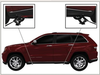
Do not raise the vehicle until you are sure the jack is fully engaged.
