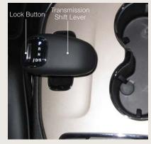
push and hold the shift lever fully forward until "P" is displayed in the EVIC.
