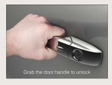
vehicle and within 5 ft (1.5 m) of the driver's or passenger front door handle, push the door handle LOCK button to lock all four doors and liftgate.
