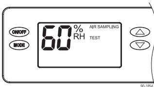
Press and hold the ON/OFF button and MODE buttons for 3 seconds. The measured humidity, AIR SAMPLING and TEST will show on the display. If wired to the HVAC system, the HVAC blower will turn on and if there is/are damper(s) wired to the DEH DAMPER terminals of the control, the damper(s) will energize.
