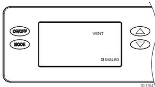
Press and hold the MODE button for 3 seconds to access the installer settings menu. Press and release the MODE button repeatedly until the VENT DISABLED screen appears.
