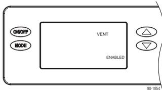
Press the UP or DOWN button to ENABLE ventilation, then press the MODE button to set Timed or Auto ventilation.
