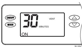
2. Press the MODE button to toggle to the VENT TIME setting.
