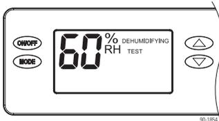
After three (3) minutes the dehumidifier compressor will turn on and DEHUMIDIFYING will replace AIR SAMPLING on the control screen.
