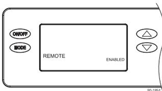
If installing in a crawl space or sealed attic with remote control, Enable and press MODE. The installer set-up is complete, proceed to **Installer Test Mode** section on page 17.
