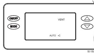
**Vent-Auto-C:** Ventilation prevented when outdoor temperature is below 0°F and above 100°F.
