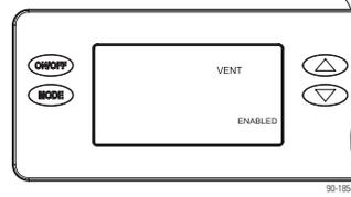
If using the dehumidifier for ventilation, Enable and press MODE to select TIMED or AUTO.
