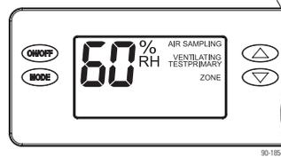
If the dehumidifier has been set up for ventilation, VENTILATING will appear on the display throughout Installer Test Mode, and the ventilation damper will be energized.
