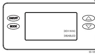
To disable dehumidification when the air conditioning is on, select DISABLED and Press MODE.
