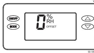
An offset can be applied to the on-board humidity reading to avoid discrepancies with other humidity measuring devices in the home. Use the UP/DOWN arrows to select an offset from -5% to 5%. Press MODE to exit the installer set-up screens.
