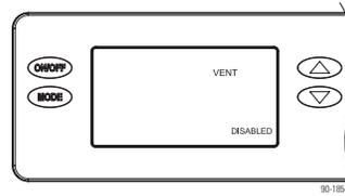
If not using the dehumidifier to bring in outdoor air, press MODE to go to ZONE screen selections.
