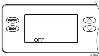
With the dehumidifier power switch on, press the ON/OFF button to turn the dehumidifier off.
