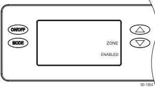
If installing the dehumidifier in a two-zone application, use the UP or DOWN arrows to select ENABLED and press MODE to go to the EXTERNAL control screen selections.
