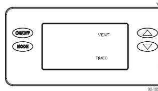
Press the UP or DOWN to toggle between VENT TIMED, VENT AUTO-B, VENT AUTO-C and VENT AUTO-D (refer to page 20 for a description of each). Press the MODE button to select the desired ventilation method and adjust the ventilation time.
