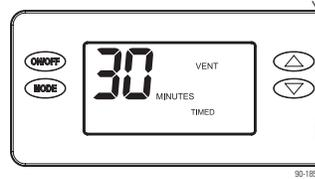
Press the UP or DOWN button to set the desired amount of ventilation time per hour from 0 to 60 minutes.
