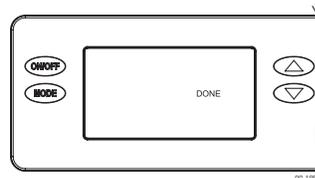
To complete, press the MODE button repeatedly until DONE appears on the display.
