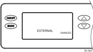
If using a Model 76, Model 8910, or Model 8620 as an external control or other third-party external control, such as a thermostat with dehumidifier outputs, use the UP or DOWN arrows to select ENABLED and press MODE to go to the dehumidification with air conditioning (DEH W/AC) screen selections.
