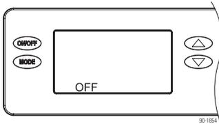
**NOTE:** If the display backlight is not on, the first button press (any button) will only turn on the backlight. Press the button a second time to achieve function.
