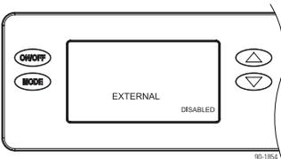
If using the dehumidifier on-board control select DISABLED and press MODE to go to the dehumidification with air conditioning (DEH W/AC) screen selections.
