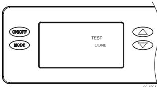
After one minute of compressor operation, all outputs will turn off and DONE will blink for 3 seconds and then return to the OFF screen.
