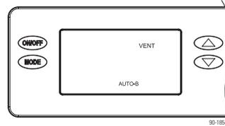
**Vent-Auto-B:** Ventilation prevented when outdoor temperature is below 0°F and above 100°F. Between 0°F – 20°F ventilation is only allowed during a HVAC heat call.
