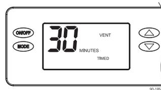
Press the UP or DOWN arrows to adjust the ventilation time per hour from 0 to 60 minutes. After selecting time, press MODE to go to the ZONE screen selections.
