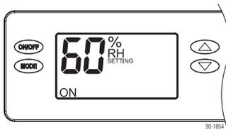
1. Press the UP or DOWN button to access the RH adjustment screen or to turn on the backlight if using an External Control.
