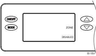
If installing the dehumidifier in a single zone application, select DISABLED and press MODE to go to the EXTERNAL control screen selections.
