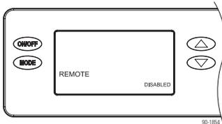
If not installing in a crawl space or sealed attic with Model 76 remote control, press MODE to go to VENT screen selections
