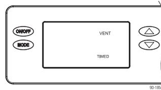
If ventilating based on time only (no outdoor temperature restrictions), press MODE at the VENT TIMED screen to go to ventilation time selection screen.
