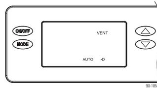
**Vent-Auto-D:** Ventilation prevented when outdoor temperature is below 0°F and above 90°F. Between 0°F – 40°F ventilation is only allowed during a HVAC heat call.
