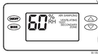
If the dehumidifier has been set up for zoning, PRIMARY ZONE will show on the display for the first minute of dehumidifier blower operation. After one minute, SECONDARY ZONE will show on the display and the zone dampers will de-energize.
