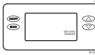
To allow dehumidification during active air conditioning, select ENABLED and press MODE.
