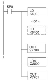
Loads a constant that specifies the number of channels to scan and the data format. The upper byte selects the data format (i.e. 0=BCD, 8=Binary) and the number of channels (set to 4 for the F0–04AD–2).
