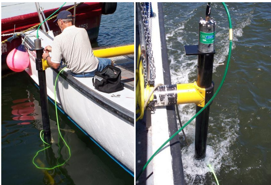
Figure 4-2: 6205 Deployment, Option 2 – Over-the-Side
