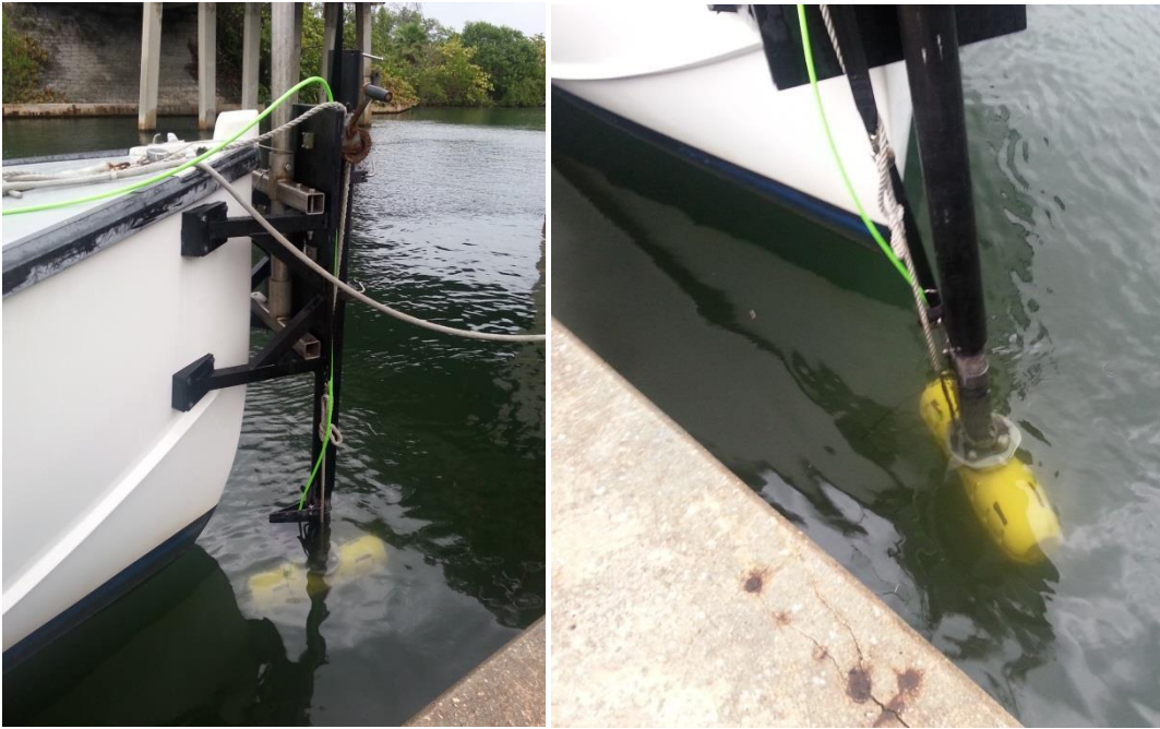
Figure 4-1: 6205 Deployment, Option 1 – Over-the-Bow
