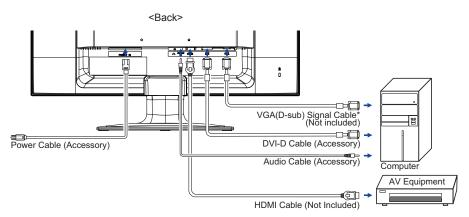
\* VGA (D-Sub) cable is not supplied with the monitor; you need to use a special VGA (D-Sub) cable dedicated for this model. Please contact the iiyama Support Centre in your country if you wish to connect the monitor via the VGA input.
