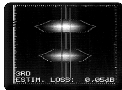
Hot image of depressed cladding fibers
