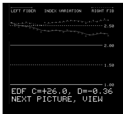
An example of a graph when the RTC procedure is initiated just after the index profiles have diverged.
