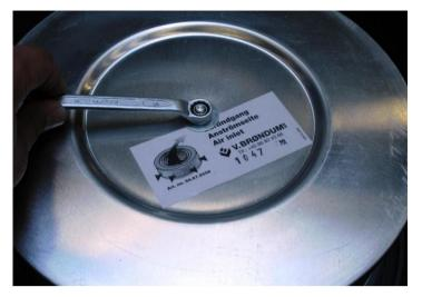
Remove the nut and washer fastening the HEPA filter. Use a size 10 ring spanner.
