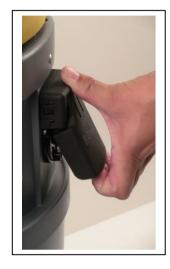
Pull the flap of the shock valve while the machine is blocked and running. (Do not tug the valve)
