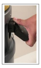
When the power grows bigger than the influence from the vacuum, the valve will automatically open with a "puff". Let go of the valve.
