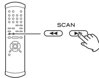
When playing back, use the SCAN button (◀◀ or ▶▶) to move backwards and forwards. Press PLAY to restart playback at normal speed at the desired location.
