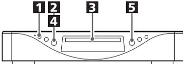
**1 Press the STANDBY button to turn the unit on.**
