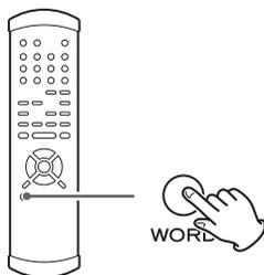
This feature is used when you want to get your whole system locked to a single sync signal (clock) by connecting this unit to the Esoteric AZ-1 or G-0/G-0s or other devices that are capable of outputting a sync signal (word clock).
