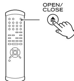
Pressing OPEN/CLOSE opens the tray if it is closed, and closes it if it is open. When the tray is opened during playback, it may take a few seconds before the disc is "unloaded" and the tray opens.
