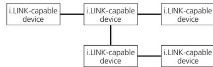
Your system does not work if data is fed back to the output device. Be careful not to create a loop.
