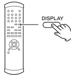
During playback, it is possible to change the display as shown here.
