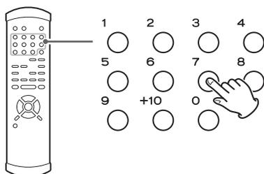
Use the number button to select tracks for playback. Use the +10 button to enter the first digit of numbers greater than 9 (repeated presses show 1-, 2-, 3- etc.) and the single digit buttons (0 through 9) for the second digit, or single-digit track numbers.
