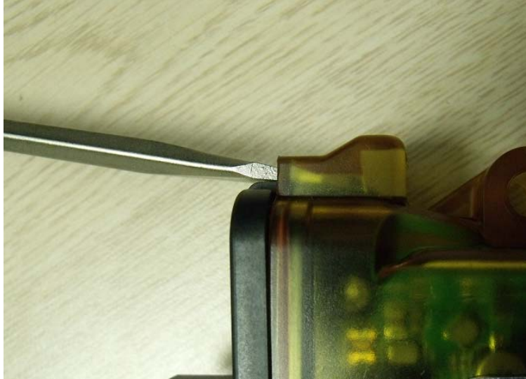
Figure 06: WIC-2402 housing removal procedure
