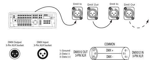
For installations where the DMX cable has to run a long distance or is in an electrically noisy environment, such as in a discotheque, it is recommended to use a DMX terminator. This helps in preventing corruption of the digital control signal by electrical noise. The DMX terminator is simply an XLR plug with a 120  $\Omega$  resistor connected between pins 2 and 3,which is then plugged into the output XLR socket of the last fixture in the chain. Please see illustrations below.
