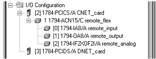
The tags created for the remote device (1794-ACN15 in this example) depend on the communication format you select for that device when you add the device to the I/O Configuration folder.
