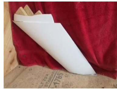
The six wooden blocks, wooden strips, and resin have been added to increase strength, reduced the amount of resin, and get the weight right.
