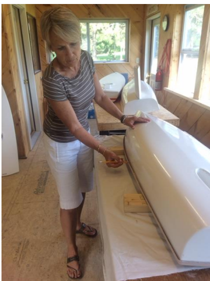
Hold the deck firmly to the hull and Pencil a nice line around top of hull.
