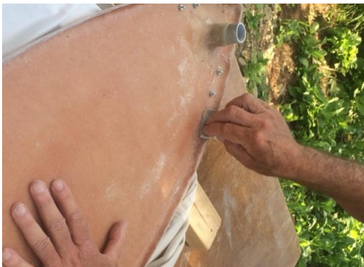
Sanding the inside of the deck flange & bottom of the deck
