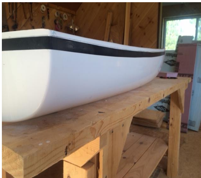
Tape just below the pencil line & then you'll know you have the deck down tight to the hull. Then sand thoroughly above the line.
