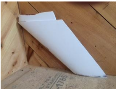
This keel has 5 cups of sand mixed in resin inside and has been set aside to cure.
