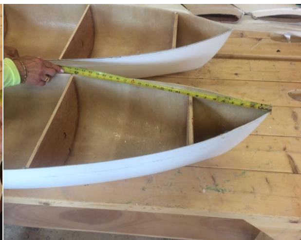
The second bulkhead should be approximately 25" aft of the stem. We no longer use a forward bulkhead which is shown in the bow of the above photo.
