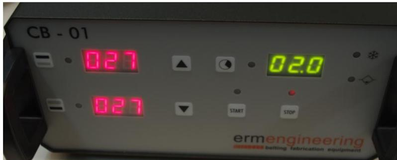
To see the temperatures assigned, it shall suffice to press the relevant button for each plate.
