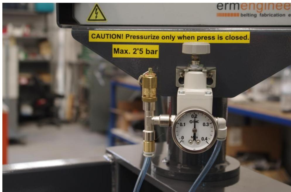
We control the inflation visually using the manometer.
