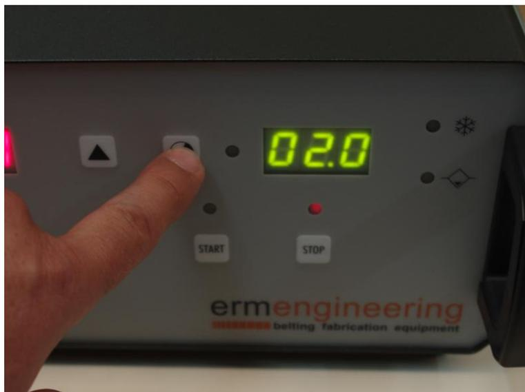
That welding time shall always show the programmed value, except for starting the count, that shall show the count-down until ending.
