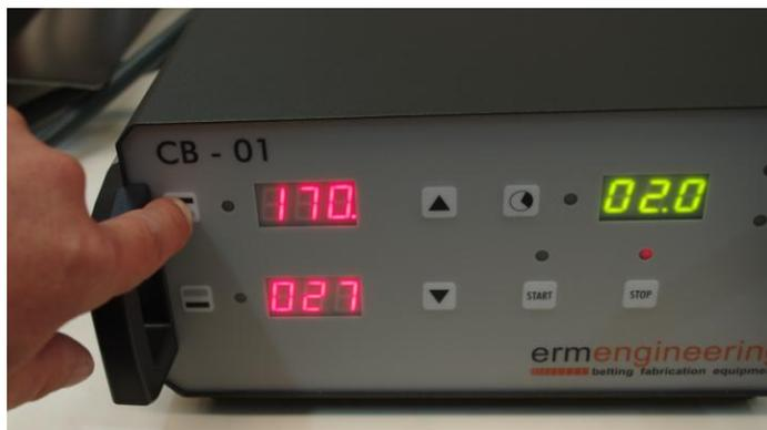
To change these values, we must hold down the button for 3 seconds and change the value using the central keys.
