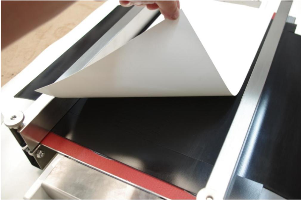
Before closing the press, we place the metal or fibreglass plate, according to the material to be welded, to avoid marks caused by the radical change of temperature and pressure outside the welding zone.
