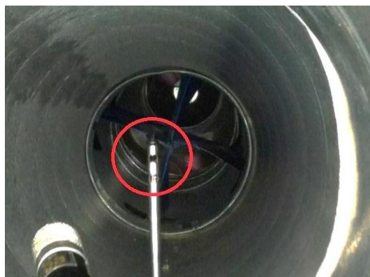
Figure 2 - Visually inspect the hotwire anemometer
