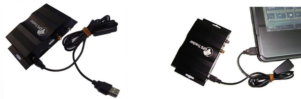
2. Connect the configuration cable with PC, open device management of your computer, you can find "Prolific USB-to-Serial Comm. Port", as following picture shows.
