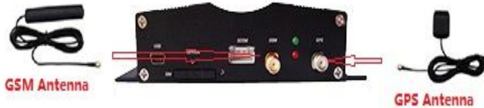
Note: Do not shield or cover the GPS Antenna with any objects containing metal.
