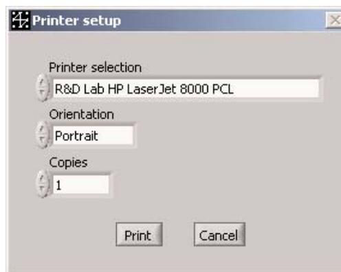
Printer and print orientation selections can be made either by clicking on the up/down buttons located to the left of the respective fields to scroll through the available choices, or by clicking in the field to produce a pop-up menu. Select the number of copies by using the up/down buttons located to the left of that field.
