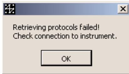
Check that the cable between the Ettan IPGphor II Isoelectric Focusing Unit and the PC is connected properly. Communication can be confirmed by selecting “Report” or “ID” from the Run drop-down menu.
