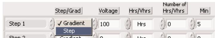
In the VHrs mode, the dialog will change slightly as the two fields (hrs and minutes) are not required to program this step. Only the total VHrs for that step will be entered.
