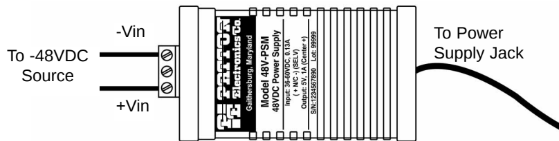
Figure 9. Connecting DC Power to the 48V-PSM DC Power Supply.
