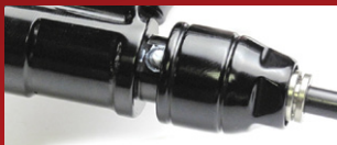
ASA adjuster in OFF position. Air will not flow.
