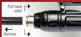
ASA adjuster in ON position. Air will flow.
