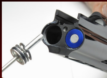
NOTE THE LPR PISTON SPRING STACK ORDER
