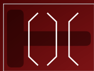
NOTE THE LPR PISTON SPRING STACK ORDER
