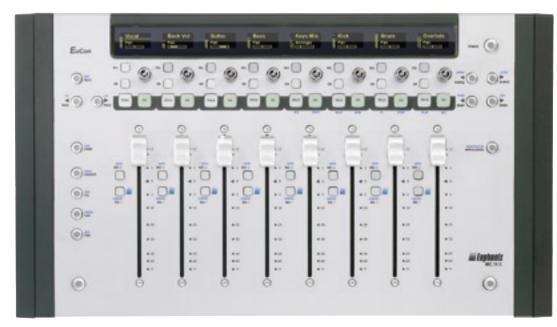
set up to be controlled. Page keys move between parameter pages in plug-ins. Like most controllers, the four faders are a window looking at a much bigger console. This window can be moved one strip at a time with Nudge keys or four strips at a time with the Bank keys. Shifted, the Bank keys move the window to the far left (home) or right (end) of the mixer. Nudge Left Shifted toggles the Mixer window and Nudge Right closes any open window or dialog.
