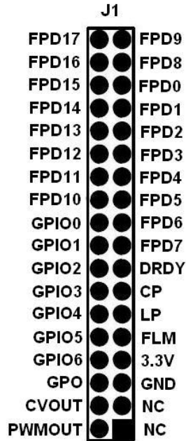
Figure 3-4 J1 PIN Configuration
