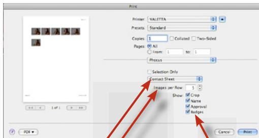
1. Check **Contact Sheet**. Select the required layout in **Images per Row**. Check boxes to include information.
