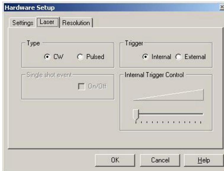
Figure 26 Hardware Setup - Laser Tab Selected
