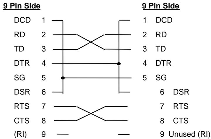
Figure 64 Null Modem cable
