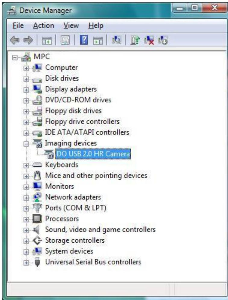
Figure 24 Drivers installed list (DO USB 2.0 HR Camera)
