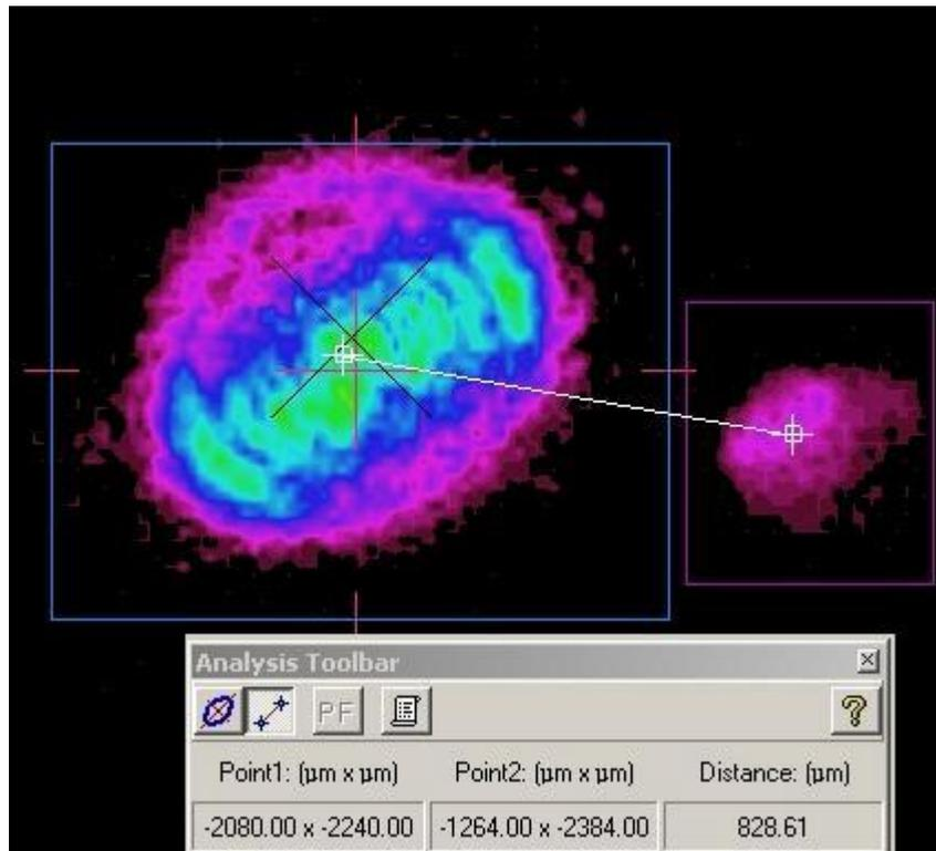
Figure 54 Measuring Distances Between two Points
