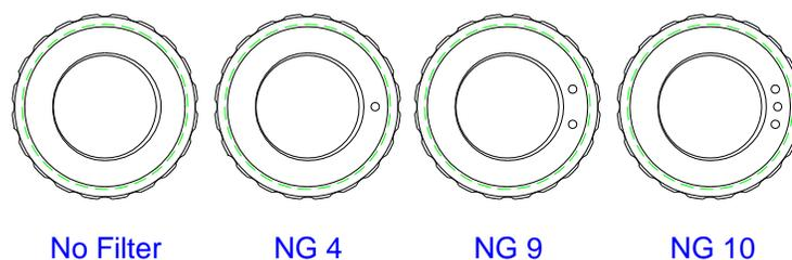
Figure 34 Filter type marking
