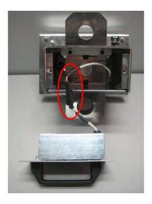
4) Unplug the connector automotive AMP from the battery pack.
