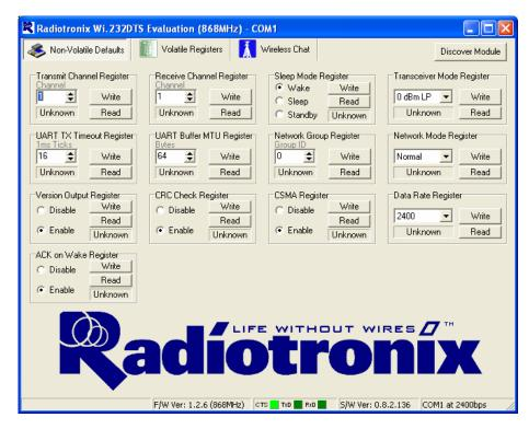
The Non-Volatile Register page in the evaluation software allows you to change the default settings which will be loaded when the module is powered on. It is important to note that data rates in excess of 19.2kbps cannot be achieved in LP mode due to bandwidth limitations.
