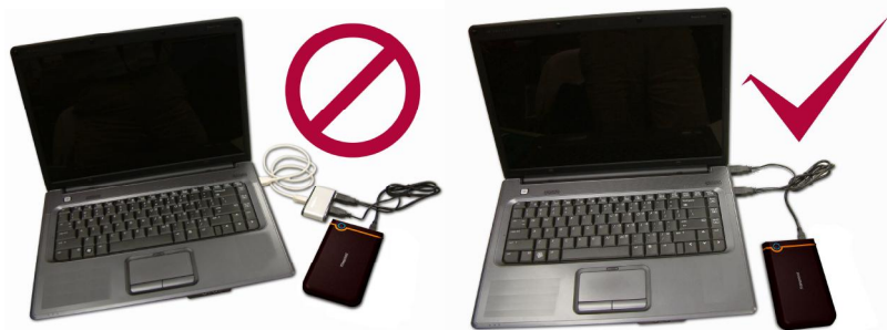
Figure 17: Plug in both USB connectors directly to your computer
