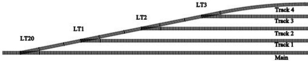
The entry to the yard from the main is controlled by Switch 20: Closed for the main and Thrown for the ladder. Switches on the yard ladder are Closed for the ladder and Thrown to select their specific track, so Switch 1 is Thrown for track 1, Switch 2 is Thrown for track 2, etc. Suppose we wish to fully line the route from the main to any yard track by only issuing one Switch command.
