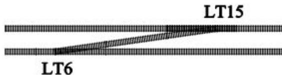
For the normal routes, both 6 and 15 are Closed. For the crossover route, both 6 and 15 are Thrown. Now suppose we want to just send Switch 6 Closed and Switch 6 Thrown to select the routes.
