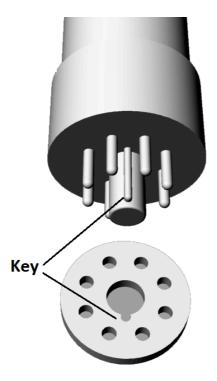
12AT7 / ECC81 tube has one missing pin acting as a correct positioning key. Align missing pin with the missing hole in the tube socket while inserting.
