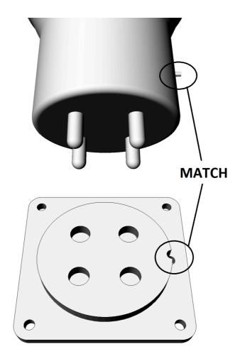
EL34 tubes have a small bump in the center as a key for correct positioning. Align it with the corresponding notch in the tube socket while inserting.
