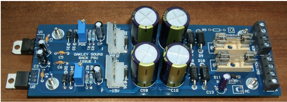
A completed RPSU board built in full wave rectification mode and fitted with Molex KK headers
