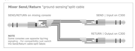
Type 1 and Type 2 cables are used when C300 is used as channel insert effects with mixing consoles that has unbalanced insert points on 1/4" stereo jacks.
