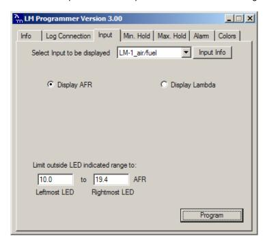
You can select the input channel to display, whether Lambda or AFR is displayed (when selecting a wideband Lambda/AFR channel) and also you can set the range of the analog 'needle' LEDs. Press the program button when you are finished.
