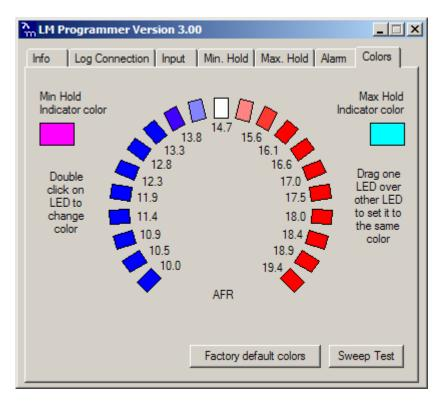
This shows the current color settings for all the 21 LEDs plus the indicator colors used when reviewing Min/Max hold
