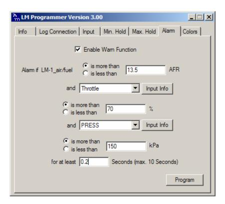
Again, the programming is very similar to the Min/Max hold programming as described in 4.6. Except here the Alarm condition can be programmed to be dependent on two other channels and time. During an Alarm the XD-16 will flash the indicated value and the analog needle LEDs at maximum brightness until the Alarm condition goes away.
