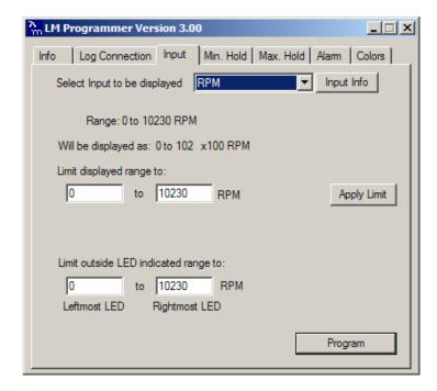
As you can see here, the display will indicate in 100 RPM. This might be too coarse for many applications. The limit is there because the XD-16 can only display 3 digits. By applying a limit (for example to 0...9990 RPM the XD-16 can display the RPM in multiples of 10 RPM. If a channel is selected that has both positive and negative values, a different screen will show:
