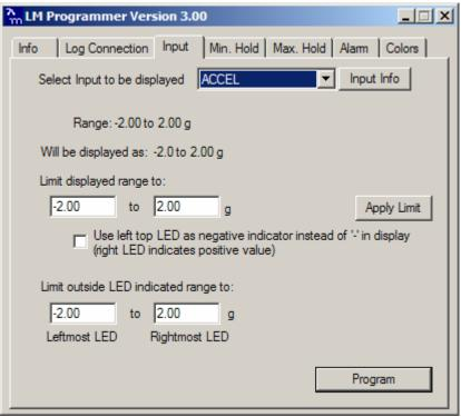
This allows you to use the Indicator 1 and 2 LEDs as negative value indicators to preserve the 3-digit resolution of the XD-16.
