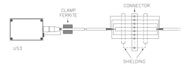
3. The CLAMP ferrite provided with the equipment must be applied to the cable.
