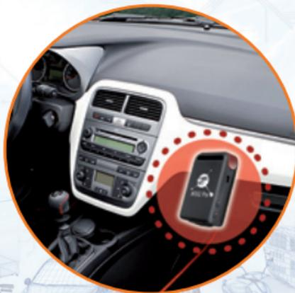
As antitheft system, it is possible to place it beneath the surface of the dashboard, inside bodywork parts of plastic, fibreglass or the like. Satisfactory results can also be achieved in other locations: under a seat, in the glove compartment, under the parcel shelf, bumper fasciae, inside aerodynamic spoilers and wing mirrors.
