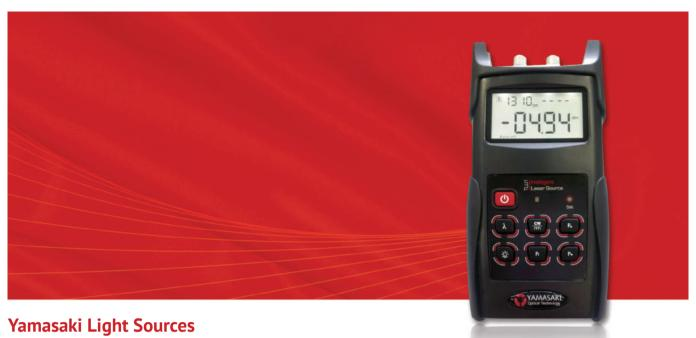
The Yamasaki TLU Series Intelligent Laser Source is the latest design in Multiple Wavelength Fibre Optic Light Source technology. The available wavelengths include 850,1300nm for Multimode and 1310,1490,1550nm and 1625nm for Singlemode. It can Generate Wave ID and Tones and the output power is easily adjustable.
