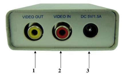
\* Be sure that you have to disconnect the [3 - Power Input] before plug-in and plug-out the SD CARD for the prevention of SD CARD damage.
