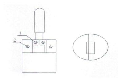
Schematic diagram of lamp and light spot on the entrance slit of the monochromator.
