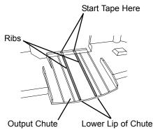
on down to the lower lip of the Chute to reduce friction and cause the discs to eject properly.
