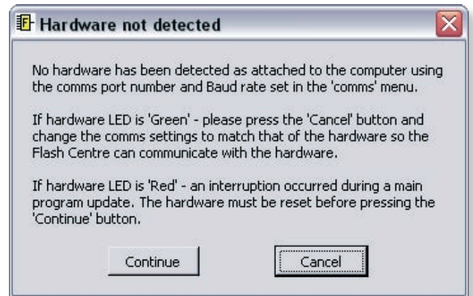
Figure 22 – “Hardware not detected” message
