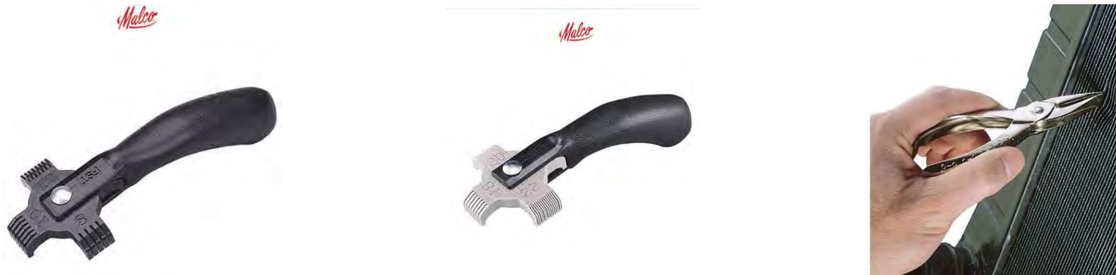
Figure 5-13: Condenser / Evaporator Fin Repair Tools (L-R) FST (for 8,10,12,14 Fins per Inch), FST2 (for 16,18,20,22 Fins per Inch), Straight-nose Pliers
