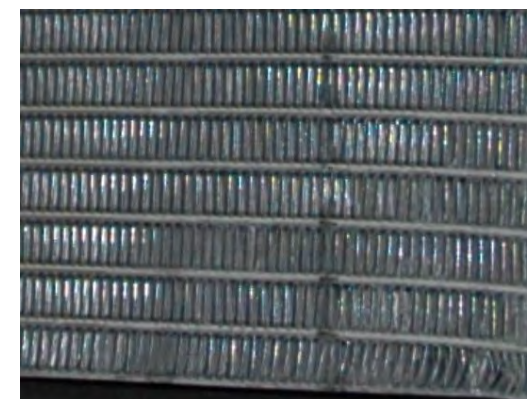
Figure 5-12a: Finned Condenser - Deformed Area
