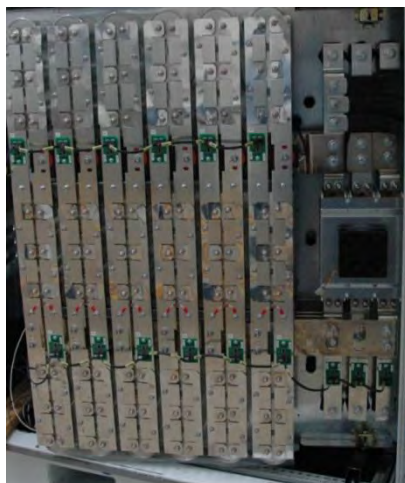
ACCESS COVER #3: AC Filter Capacitors and Contactor
