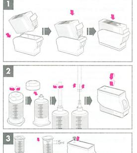
**1.** Insert the cartridge into the refill clip completely. Place the sponge side of the cartridge first and then press down the opposite side **until you hear it clicking into place.**
