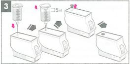
**3.** Insert the ink injection needle into the hole of the refill clip tank, and inject **5ml of ink. Wait 1 to 2 minutes** until the ink is completely absorbed into the sponge inside the cartridge, and then close the hole again **with the supplied rubber plug.**
